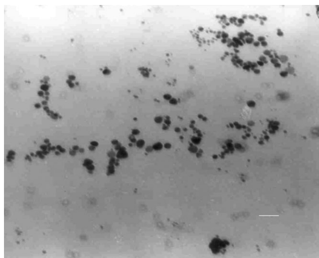
Figure 9 TEM images of the Ag clusters formed upon irradiation in aqueous GG solution (bar length = 100 nm).
